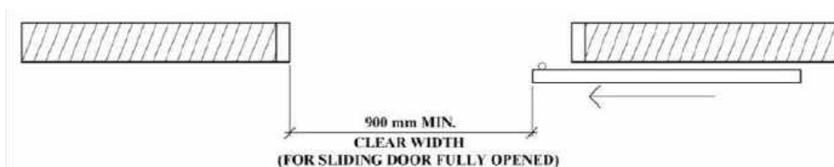
Figure 33. Image above shows a sliding door with a minimum clear opening of 900 mm
